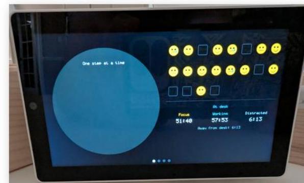
Desk display: M5Stack Tab5 (ESP32-P4, camera). Time, a face for each finished sheet, focus and away time
